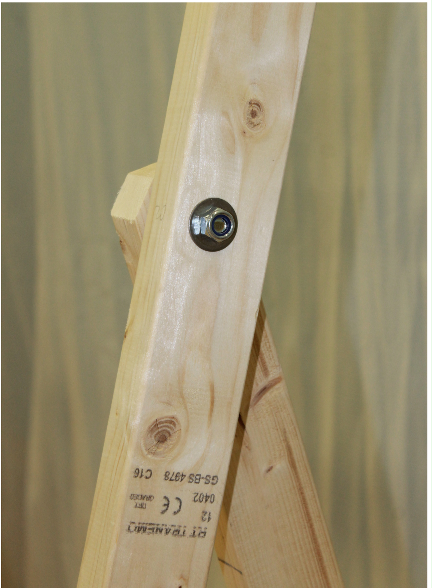
Joint between front & back legs - top of back leg must be chamfered so that it does not interfere with the boss.
