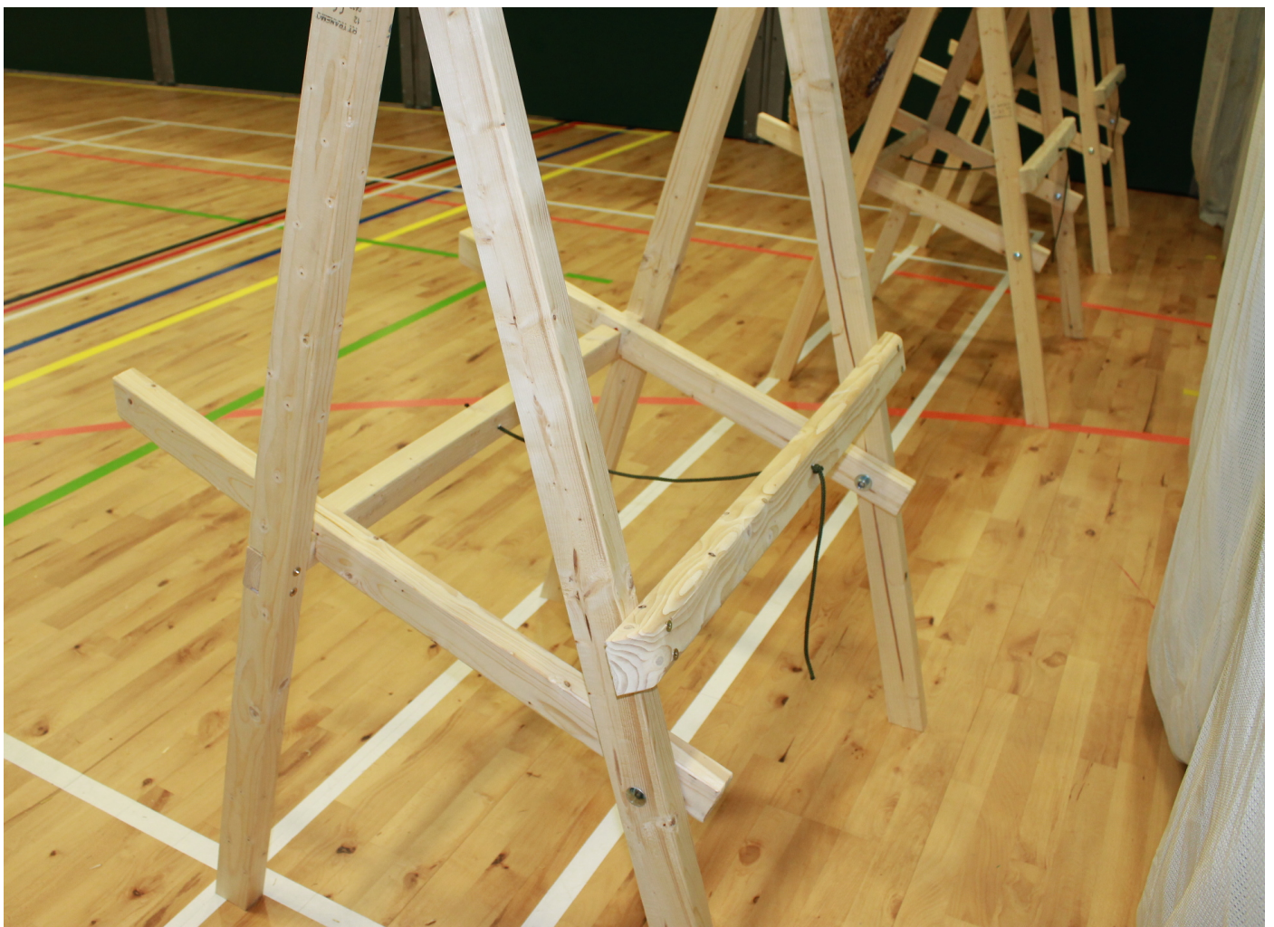
Several complete stands, note the safety cord which is not meant to be taut - the support arms define the exact angle.
