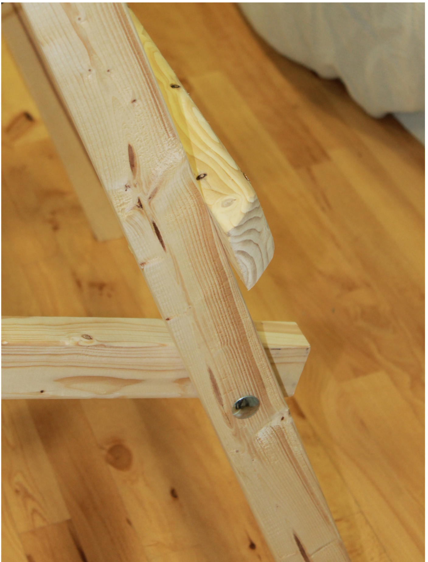
Detail of rear cross bar, rear leg, and the rear of the support arm. Note that the head of the coach-bolt is very low profile, and much less likely to damage an arrow than a conventional hex-head bolt.
