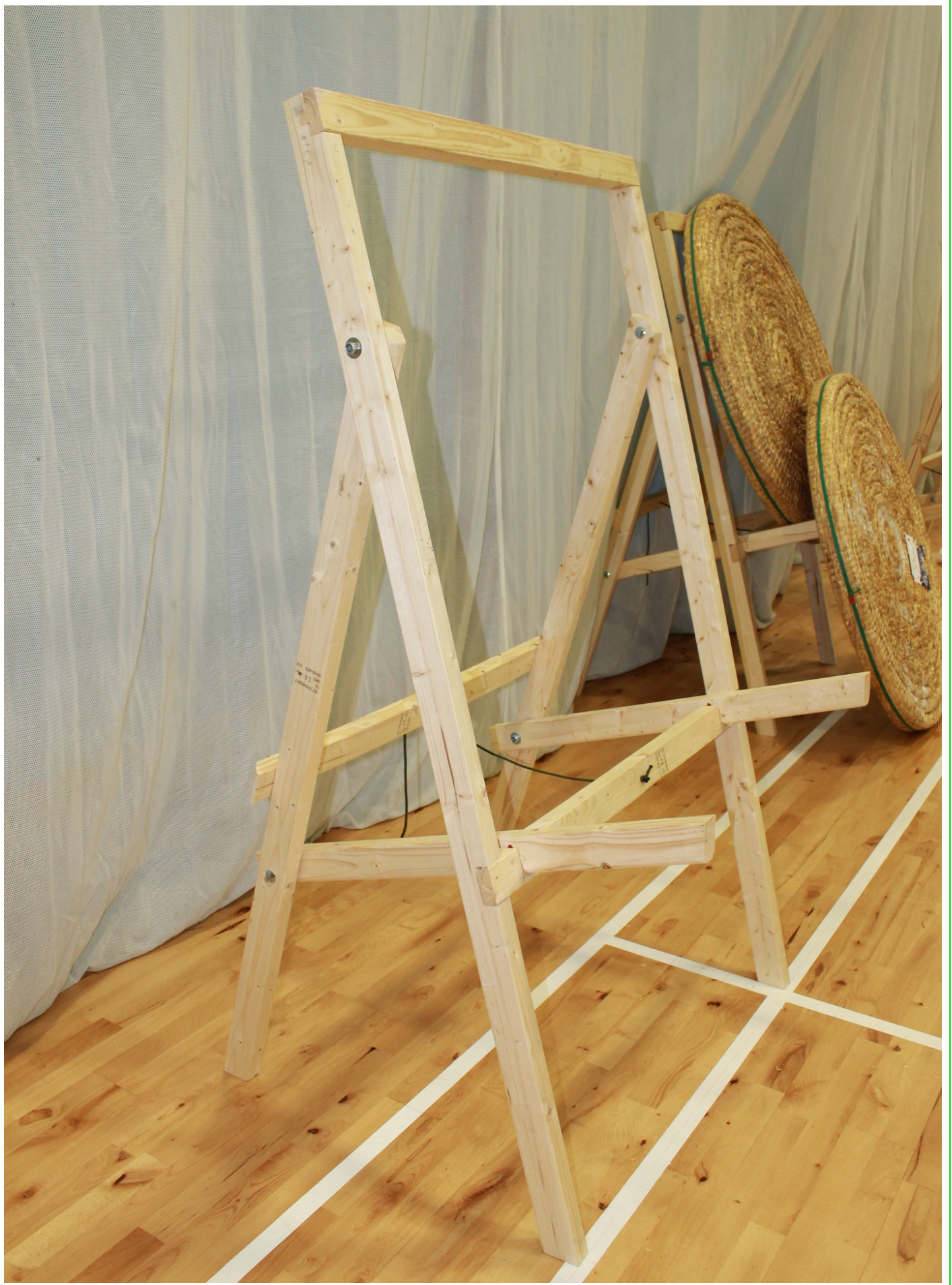
General view of full stand. Note how the rear cross bar is slightly wider than the rear legs, to match the front legs when folded.
