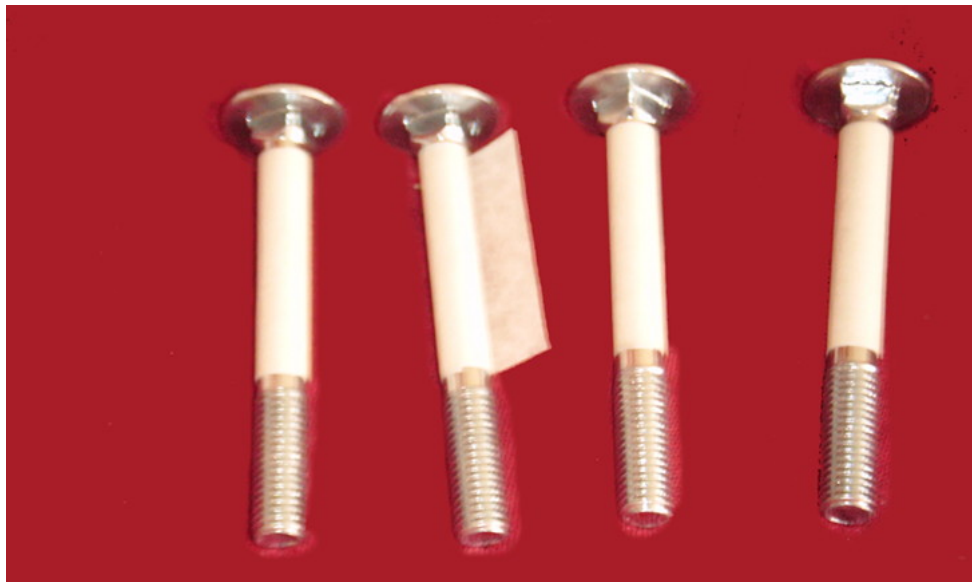
Bolt shafts wrapped with masking tape to correct diameter
