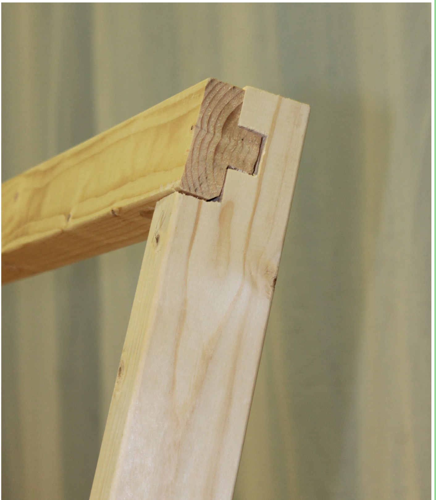
Detail of top cross bar joint to front leg - a simple lap joint will speed up construction time considerably, at the cost of a slight decrease in rigidity.
